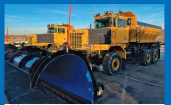
(2) 2005 Oshkosh Model P/MPT Series Sand Trucks w/ Hi-Way Hydraulic Salt Spreader Conveyor Bed & Spinner
