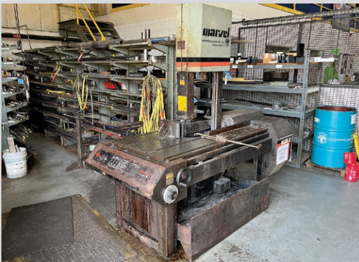
18" Marvel Series 8 Mark II Tilt Frame Vertical Band Saw
