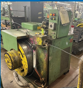
3/8" National 68 High Speed DSSD Cold Header
