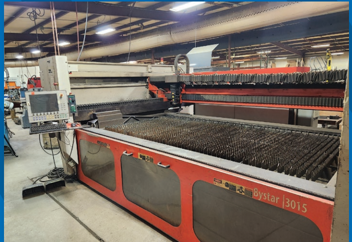
4,000 Watt Bystronic Model Bystar 3015 CNC CO2 Laser w/ 5' x 10' Shuttle Tables, Chiller & Dust Collector
