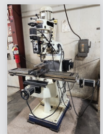
3 HP First Vertical Mill w/ DRO
