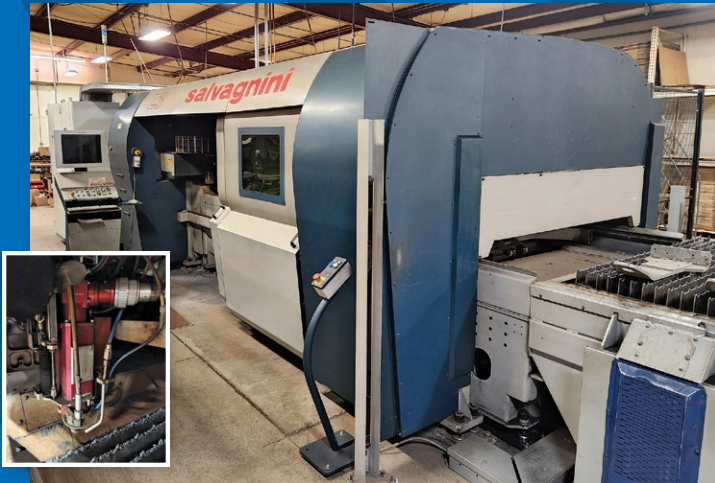
3,000 Watt Salvagnini Model L3-30.SYS CNC Fiber Laser w/ 5' x 10' Shuttle Tables, Sideros Dust Collector
